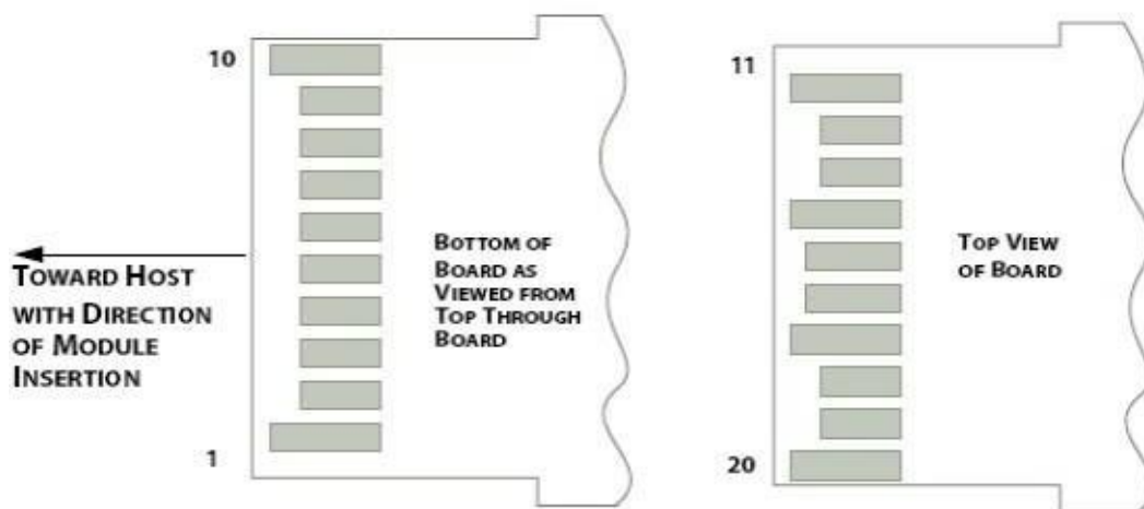
Figure 3. SFP28 Module Contact Assignment
